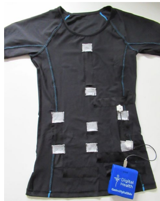
GastroDigitalShirt system with embedded microphone array and computing device won the 2019 DGVS Innovation Award "Digital Gastroenterology". The system is being evaluated in a clinical study at UK Erlangen (Baronetto et al., 2020).
